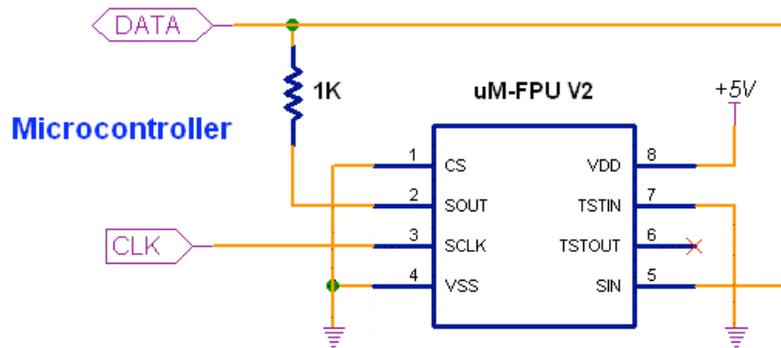
If a 2-wire SPI interface is used, the SOUT and SIN pins should not be connected directly together, *they must be connected through a 1K resistor*. The microcontroller data pin is connected to the SIN pin. See the uM-FPU datasheet for further description of the SPI interface.
